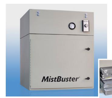
A media-based air filtration system for the collection and removal of mist, smoke and metal particles produced by machine tool operations. The system uses 58 sq. ft. of lofted micro-fine fiberglass media in its second filtration stage.
