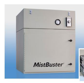
A media-based air filtration system for the collection and removal of mist, smoke and metal particles produced by machine tool operations. The system uses 58 sq. ft. of lofted micro-fine fiberglass media in its second filtration stage.
